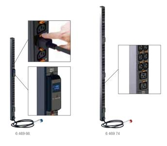
To provide  $\sim$  electric power for IT equipment in 19" enclosures 32 A PDUs are equipped with hydraulic magnetic circuit protection with high current interruption capacity. Hydraulic magnetic circuit breakers are not affected by ambient temperature
